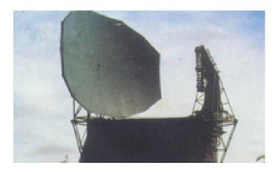
Sensors / EW: - China JY-8 Wall Rust - Radar, Radar, Air Search, 3D Long-Range, Max range: 351.9 km
