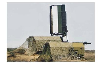
Sensors / EW: - Tin Shield A [5N59] - (ST-68M) Radar, Radar, Air Search, 3D Long-Range, Max range: 351.9 km
