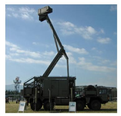
Sensors / EW: - RAC-3D - (DEHAWK) Radar, Radar, Air Search, 3D Short-Range, Max range: 100 km
