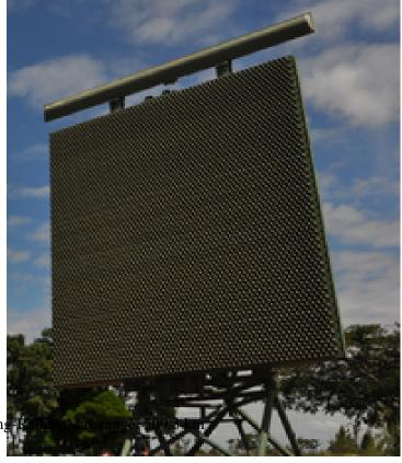
Sensors / EW: - TRS 2230 - (1979, 3D) Radar, Radar, Air Search, 3D Long
