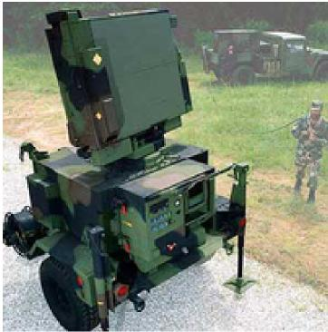
Sensors / EW: - AN/TPQ-36A - (NOAH/NASAMS) Radar, Radar, FCR, Surface-to-Air, Short-Range, Max range: 74.1 km
